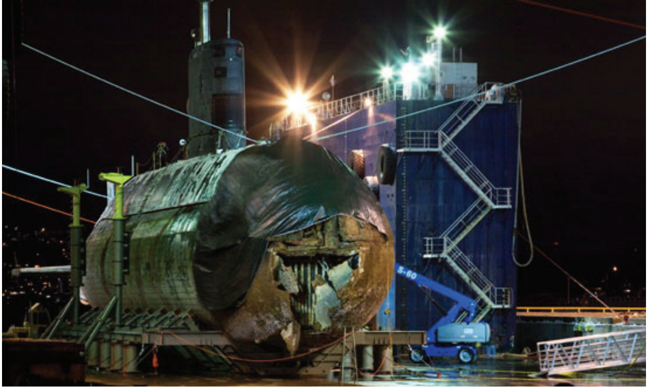
HMCS Corner Brook With Damage From Grounding
